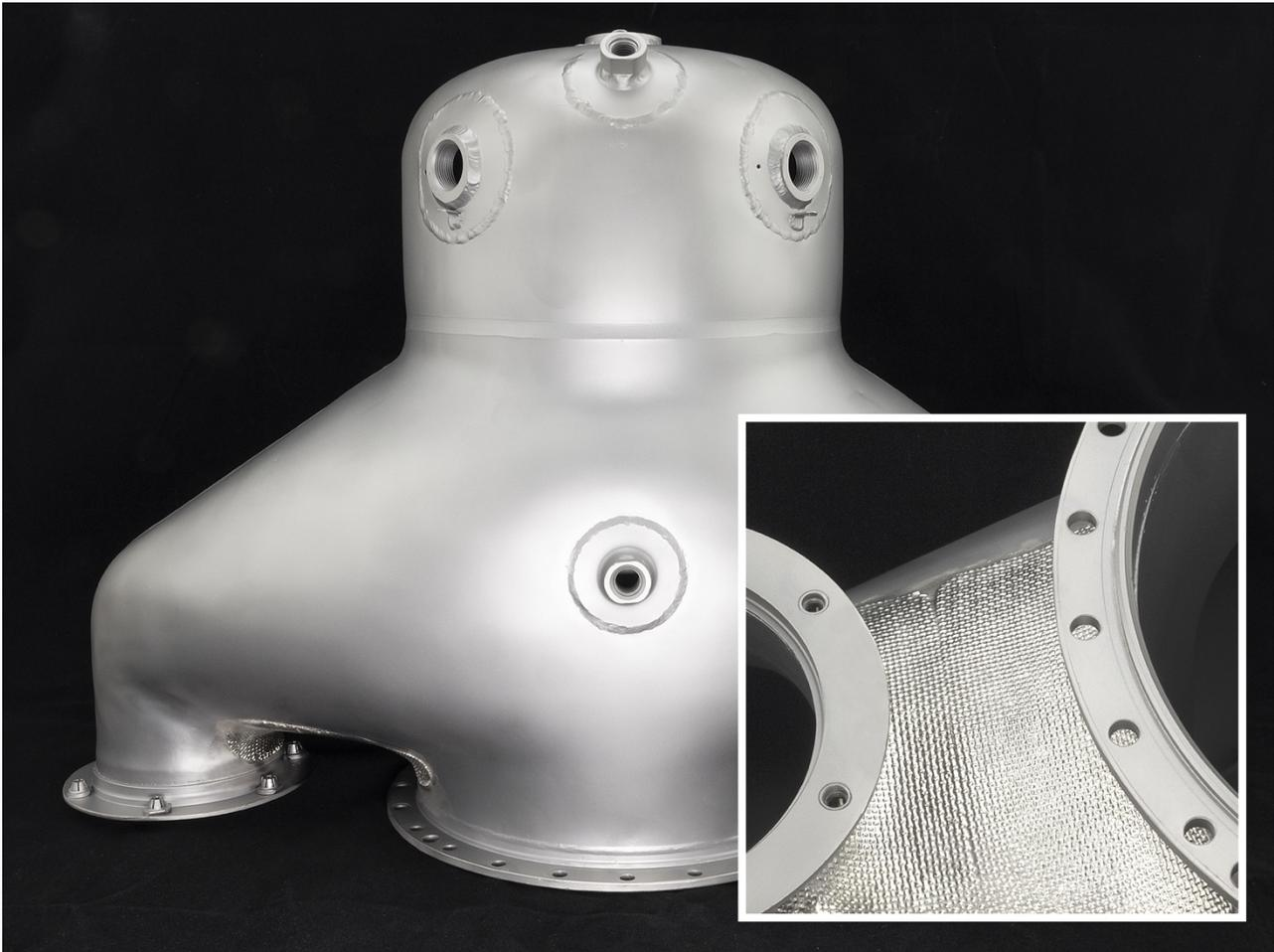
Cadorath, in partnership with Rolls-Royce, has announced the design and approval to provide repairs and overhauls to the M250 Series IV Outer Combustion Case (OCC). Overhauls will include repairs to the fuel boss and replacement of the existing wire mesh patches with new reinforced dual wire mesh patches.
