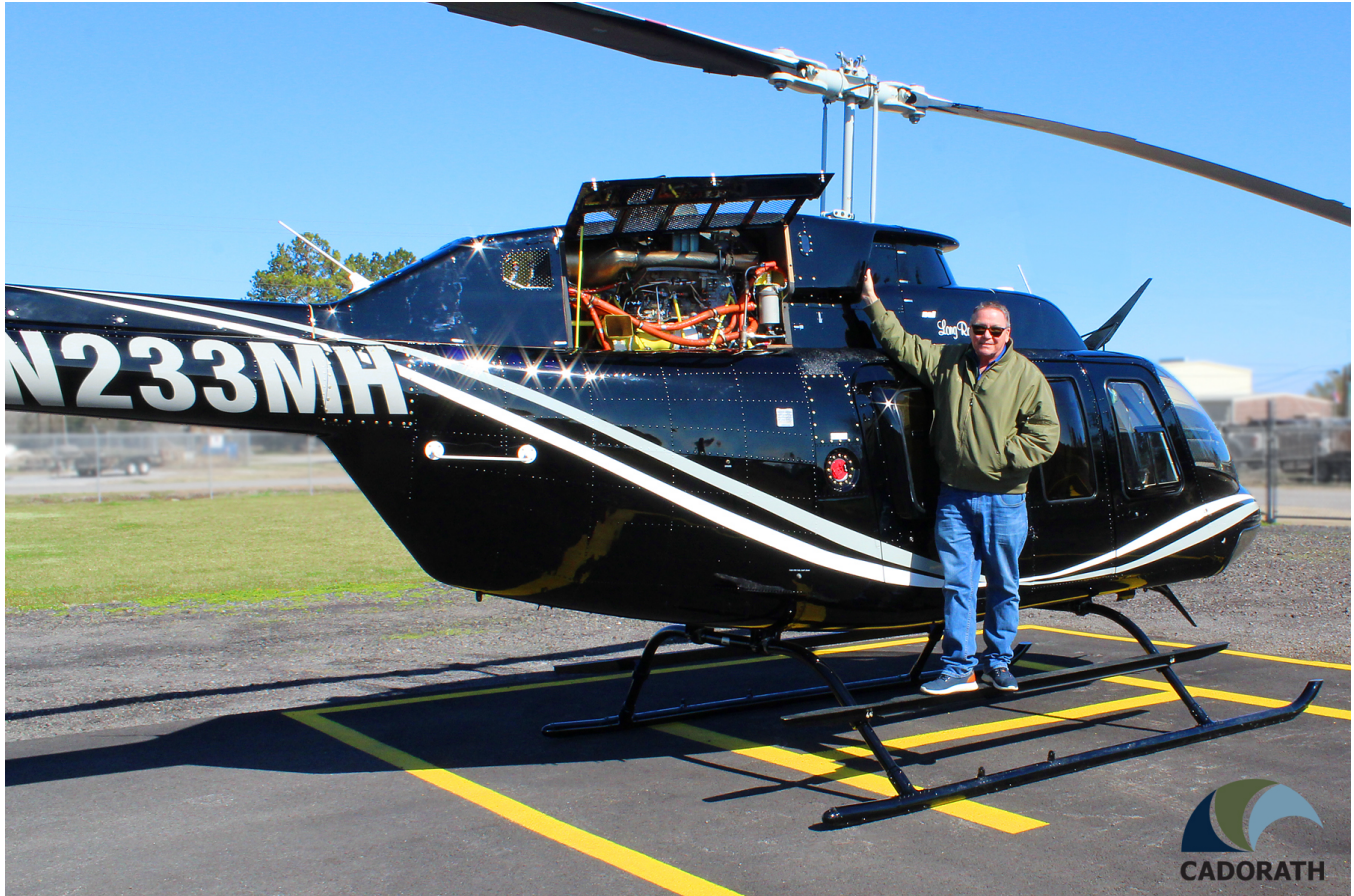
Gerry Cadorath, President and CEO of Cadorath, stands on the flight steps of a Bell 206L3, showcasing the newly overhauled Rolls-Royce M250C30P engine installed within.
